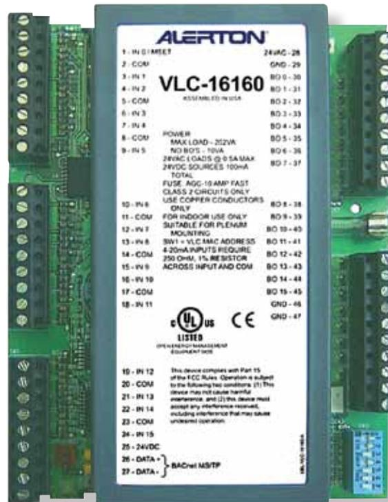
The Alerton® BACtalk® VLC-16160 is a high-performance, fully programmable logic controller designed for central plant systems, lighting panels, and other applications with numerous control points. As a native BACnet controller, the VLC-16160 integrates seamlessly with your BACnet system, communicating at up to 76.8 Kbps on a BACnet MS/TP LAN. It can also operate as a stand-alone controller.
