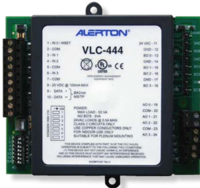
The Alerton® BACtalk® VLC-444 is a versatile, high-performance, BACnet-compliant field controller designed for fan-coil units. As a native BACnet controller, the VLC-444 integrates seamlessly with your BACnet system. It communicates at up to 76.8 Kbps on a BACnet MS/TP LAN or can operate as a stand-alone controller.
